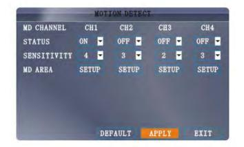
The Motion Detection Menu has 3 sections, including Channel Status, Sensitivity and Motion Area.
